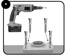
Using a power screwdriver, mount the plate to the boxspring using the supplied hardware. **Use only 4 screws per plate.**
