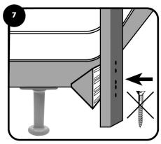
Complete installation, simply bolt the headboard onto the bracket.
