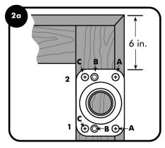
Before drilling, pick the set of screw holes you will use by measuring the width of your boxspring rail. If your rails are an actual width of  $3/4" \times 3 1/4"$ , use the outside holes [C]. The side with the single set of holes [A] always faces the outside edge of the bedframe.
