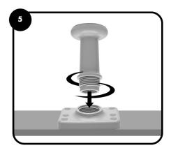
Hand twist the threaded leg stem into the base plate.
